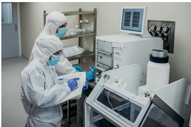
The TechnoPhage team uses the Cellexus CellMaker for its phage production. Source: TechnoPhage.
